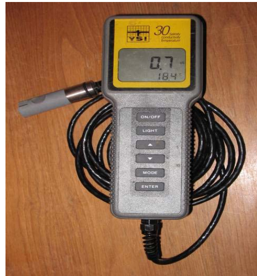
Photo2.2 YSI Model 30 Conductivity/Temperature Meter
